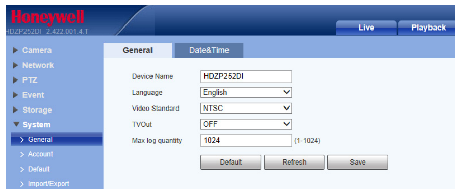
Figure 5-35 General System Configuration Interface
